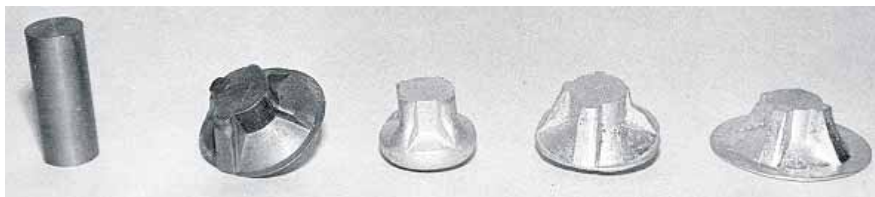
Fig. 2. From left to right: stock sample, forging made of lead, forgings made of AlCu4Mg: conventional forging (load 32kN), conventional forging (load 91kN), thixoforming (load 32kN) (W. Lapkowski, J. Mat. Proc. Techn, 80-81, 1998, 463-468)
