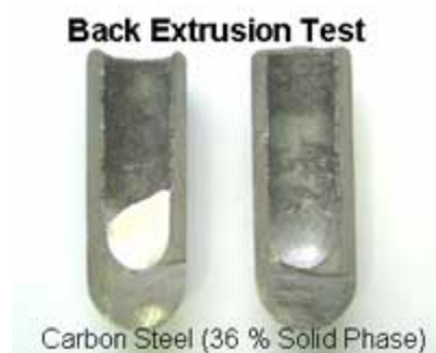
Fig. 1: Back Extrusion Test: relationship between force and position, temperature 1420 °C (58 % solids), 1440 °C (36 % solids), 1450 °C (10 % solids), velocities of deformation 0.5 cm/min.
