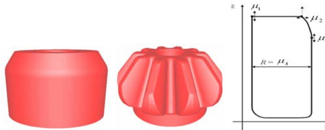
Figure 2: . Full preform and gear shapes ( not real scale ) - Parameterization of the geometry of the radial plane
