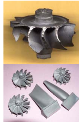
Fig. 3 Comparison of the quality of the VIM-based cheap precision casting technology from December 2001 (upper picture) and from October 2004 (lower picture)
