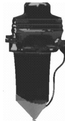
Fig. 2 Merging 3 quality criteria. Nodes showing freckle tendency are shown white, nodes of too high a curvature are shown light gray, and nodes of too low a G/v ratio are shown dark gray.
